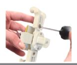
2. Insert the blue key into the axle of the Scorpion (green dot side) and rotate counter-clockwise to expand the legs wide enough for the device to fit into the Scorpion.
