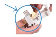
5. Press firmly on the front of the device to ensure the dual lock and leveling plate fully adheres to the device.
