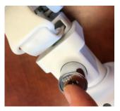
5. Align the watch with the center of the leveling plate.
