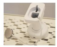
3. Take the top, and use the security key on the axel of the Scorpion and turn counter clockwise to ensure that the legs are fully extended. Once the legs are fully extended, insert the charging puck.
