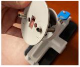
3. Align the studs with the holes in the fixture. Feed the charging cable up through the base of the Scorpion.
