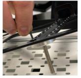
2. Use washer and wing nut to mount to fixture.
