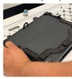
5. Secure Scorpion to plate using supplied screws (4 spots total)
