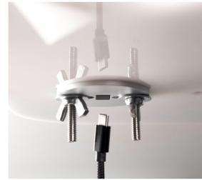
12. Place the installed device into the receiver. Press the lock in to secure. Scorpion should now be locked into place.
