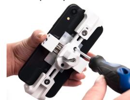
**NOTE:** 3 turns and switch until plate is raised
