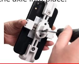
10. Secure top and bottom leg by inserting the blue key into the center of the Scorpion Body located on the back side of the device. Turn the blue key clockwise to tighten the screw and lock the axle into place.
