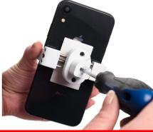
9. Feed the charging cable through before attaching Scorpion to the base.
